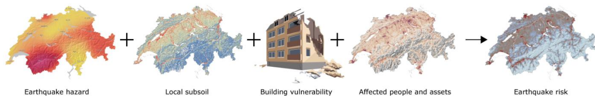
Figure 20 Components used to determine earthquake risk.
