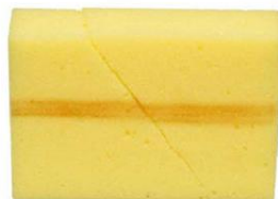
Figure 1 Normal fault, before slip. BGS ©UKRI
