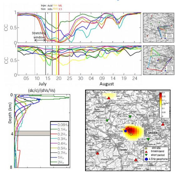
We compute noise-correlograms (NC) to construct the Greens fct. between SGTnet station pairs.
