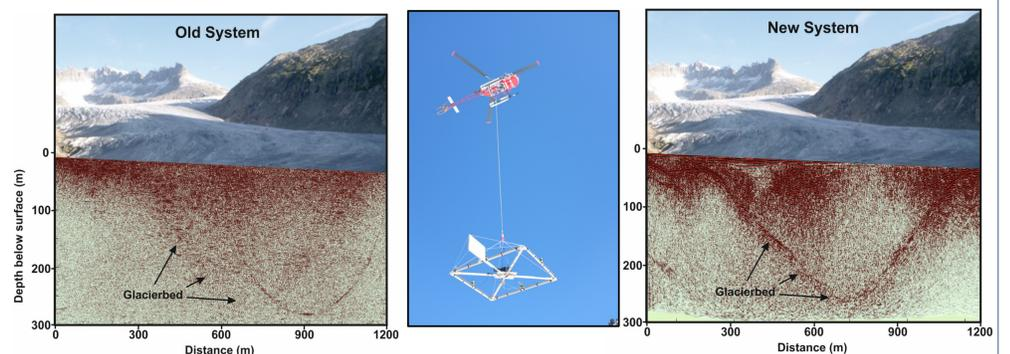
Figure 4a: Radargram across a glacier tongue using the old 67 MHz system
