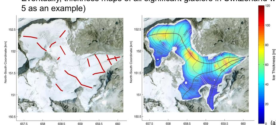
Figure 5: Radar survey transects flown on the Minstiger glacier and the resulting ice thickness map, based on Lucas (2014).
