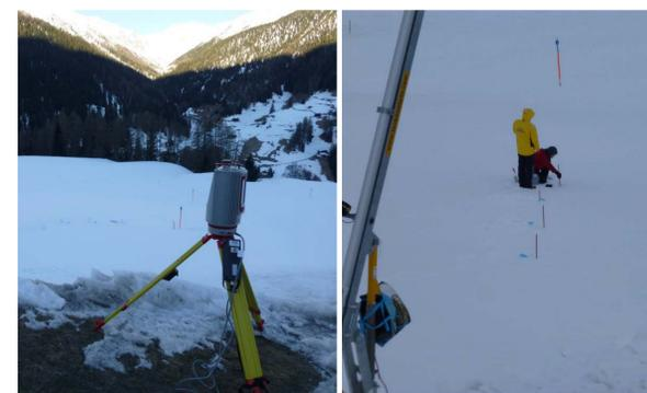
Figure 6: Terrestrial laser scanning (left) and manual snow observations (right) during snow making test
