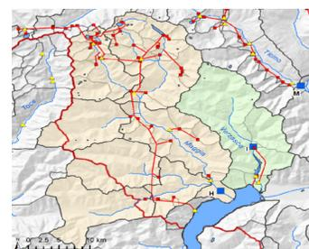
Example demonstrating the complexity of the hydraulic model structure of the model developed for the forecast of the hydro-power production in Ticino. The objective of the 3rd year will be the optimization of this power production running probabilistic extended range forecasts
