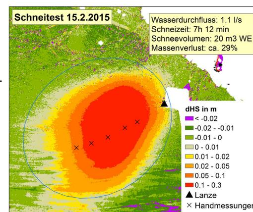
Figure 7: Result of snow making test
