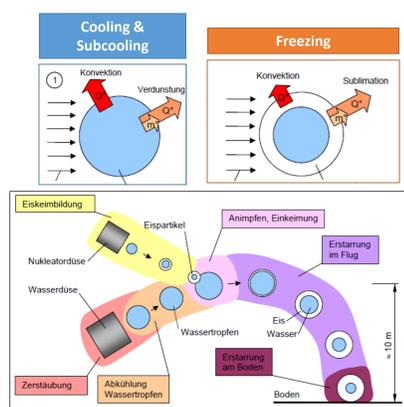
Figure 4: Physical processes during technical snow production
