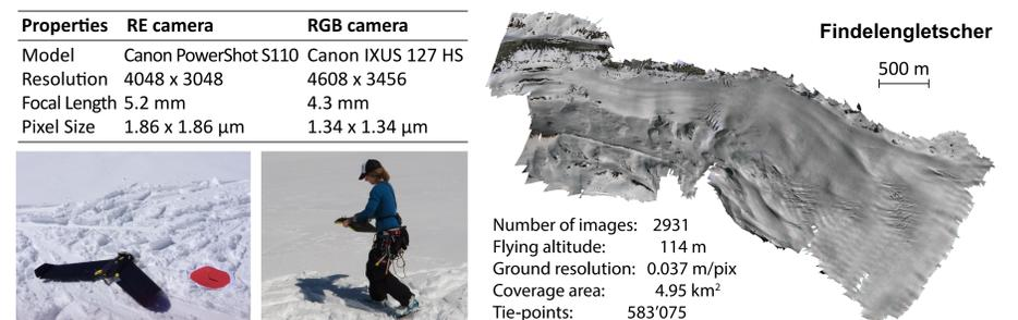
Fig. 4: Camera characteristics (table) for the UAV-system used (pictures: UAV and ground control point (left) and launching procedure (right)). An example of an orthophoto acquired for Findelengletscher in April 2015 (right) is shown. The mosaic is composed out of 10 flights.
