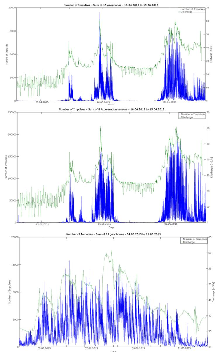
Fig. 2: Geophone sensor data for 2 months (top) and 8 days in June (bottom), and accelerometer sensor data for 2 months (middle).
