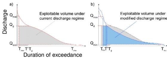
Fig. 3: Use of flow-duration curves to estimate the water volume for run-of-river HPP under a) observed and b) an assumed future discharge regime (source: Schaeffli, 2015)
