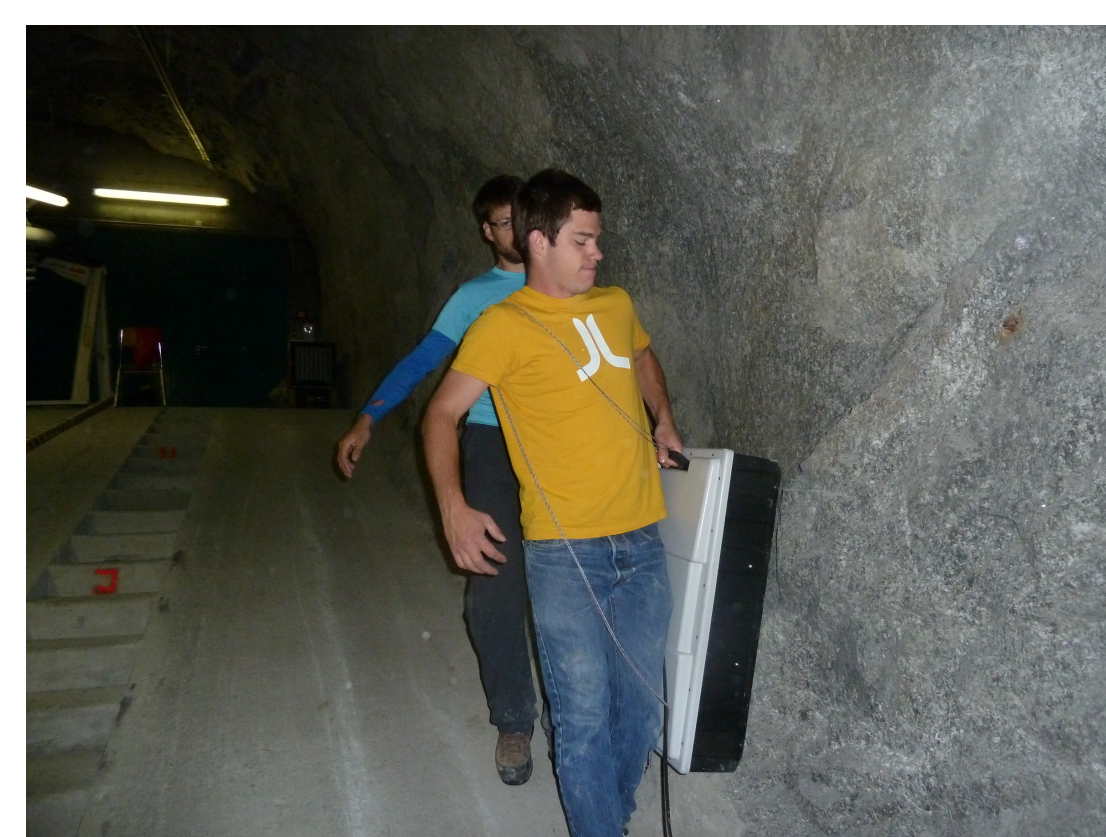
Performing GPR measurements with the PulseEKKO 250 MHz antenna (left) and the MALÅ GX HDR 80 MHz antenna (left)
