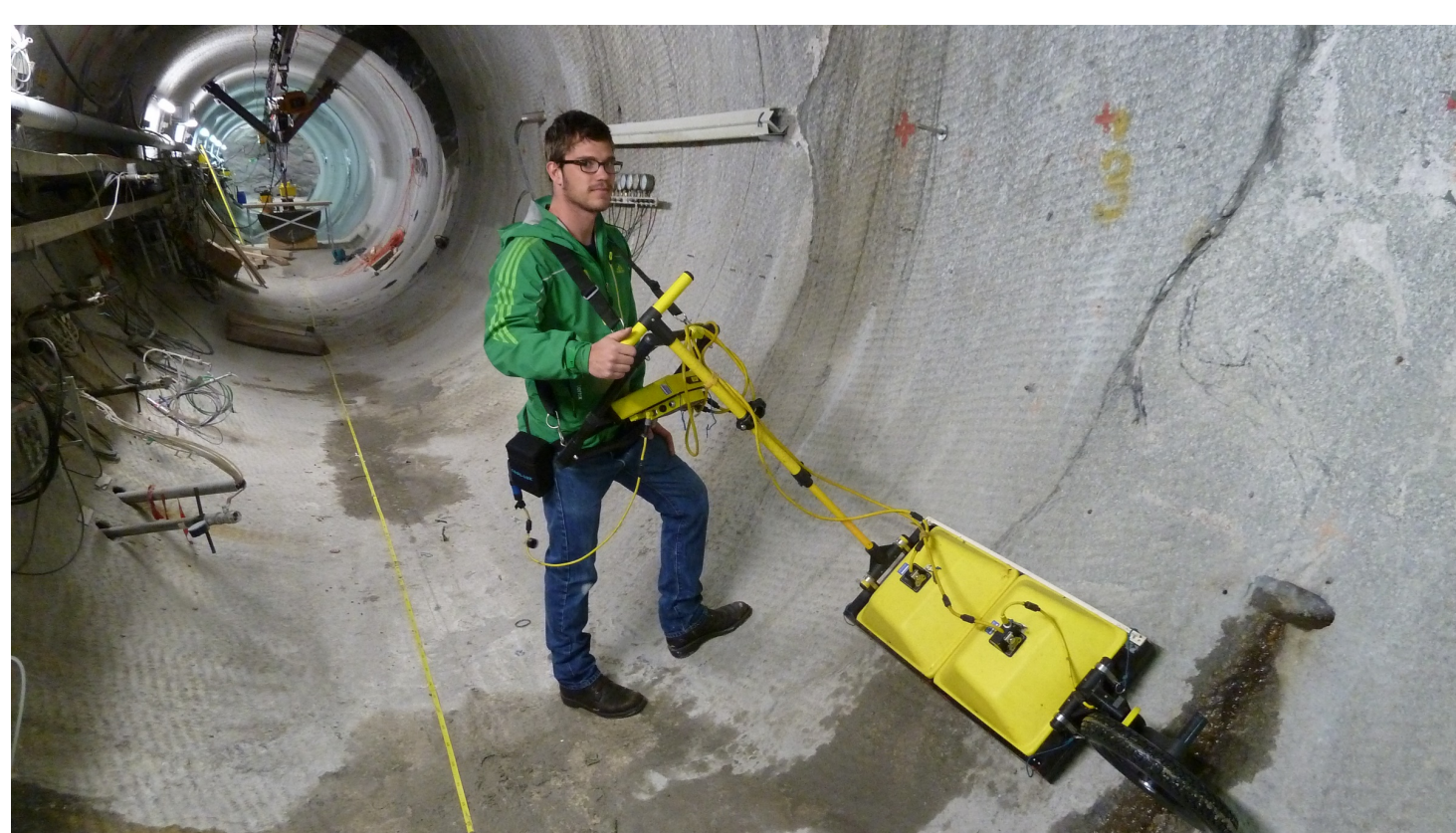
Performing GPR measurements with the PulseEKKO 250 MHz antenna (left) and the MALÅ GX HDR 80 MHz antenna (left)
