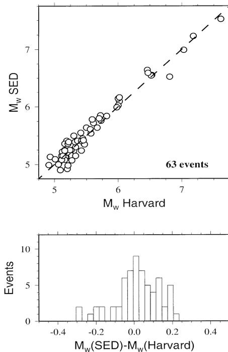
**Figure 6.2.** Comparison of  $M_w$  from Harvard CMT solutions and  $M_w$ (SED) for 63 events in the European-Mediterranean region. Top:  $M_w$ (SED) versus  $M_w$ (HRV). Bottom:  $M_w$ (SED) -  $M_w$ (HRV). Details in text.
