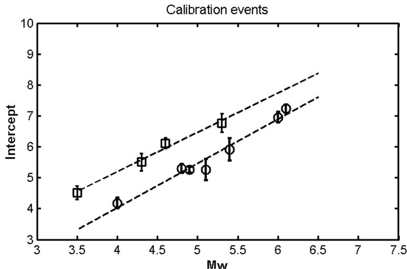
Figure 4.11. Regression of intercept intensities versus magnitude  $M_w$ . Shallow and deep events shown as squares and circles, respectively. Error bars are 1 standard error.
