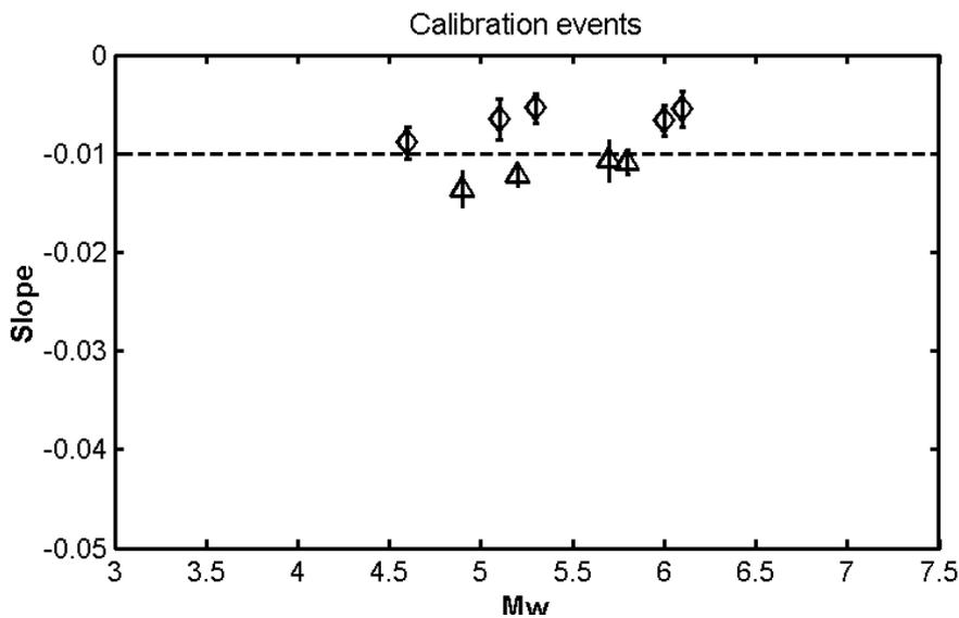
Figure 4.9. Attenuation slopes of calibration events at large distances, obtained by least squares linear fitting of mean intensities in the 70-200 km distance range. Foreland and alpine events shown as triangles and diamonds, respectively. Error bars are 1 standard error.
