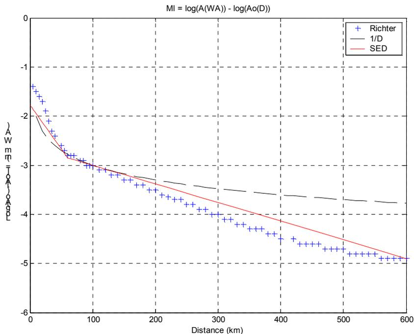
Figure 6.6. Amplitude-distance relation used for computing local SED magnitudes compared to the one introduced by Richter for California and to an attenuation proportional to the reciprocal distance ( $1/D$ ).
