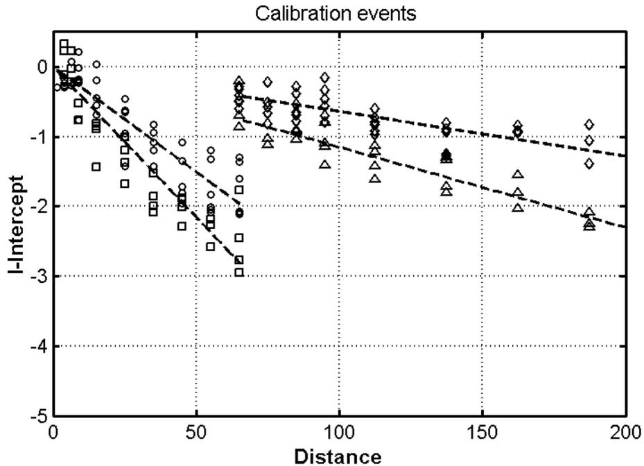
Figure 4.10. Best fitting lines for mean intensities with distance, normalized to intercept intensities, computed in the 0-70 and 70-200 km distance range. Circles, squares, triangles and diamonds represent deep, shallow, foreland and alpine events.
