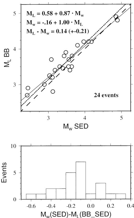
Figure 6.7. Comparison of  $M_L$ (BB-SED),  $M_L$  computed with broadband records by SED, versus  $M_w$  (SED) for 24 events in the Swiss region in the 1999-2001 period. Top:  $M_L$  (BB-SED) versus  $M_w$ (SED). Bottom  $M_w$  (SED) –  $M_w M_L$ (BB-SED). Details in text.
