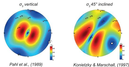
Fault reactivation pressure is lower if  $\sigma_3$  incline towards SW.
