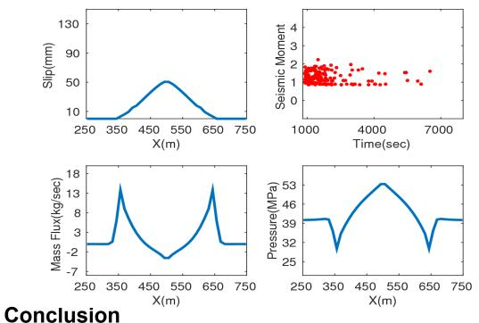
The developed volume relaxation model, stabilizes the flow solver without resolving the timescale of mechanical shear failure. As a result of this, a pressure diffusion dominiated shear failure is observed along the fracture.
