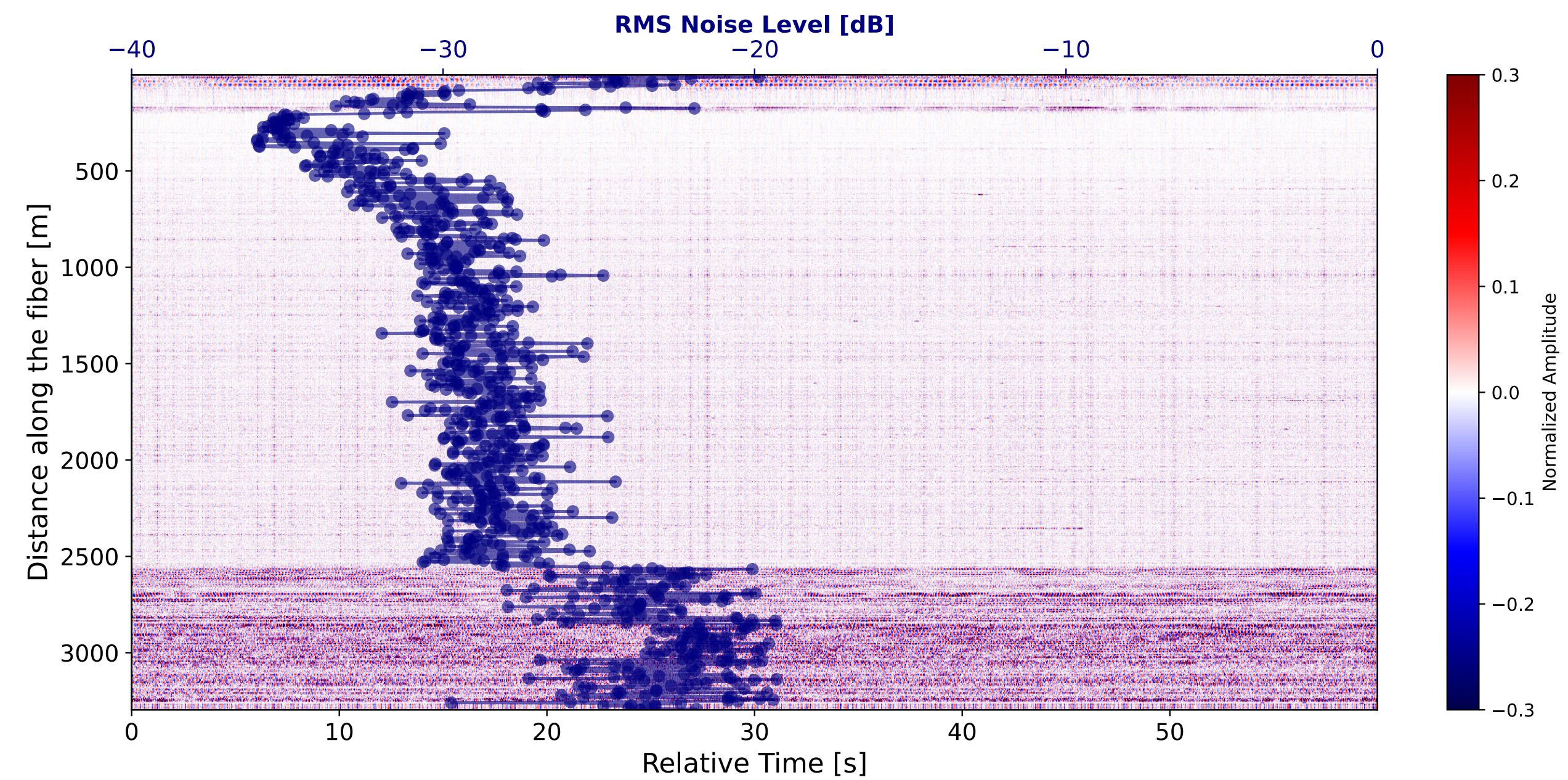
During the **pre-CO<sub>2</sub> injection** stage of the CCS project, higher noise level were observed starting from different channels over time.
