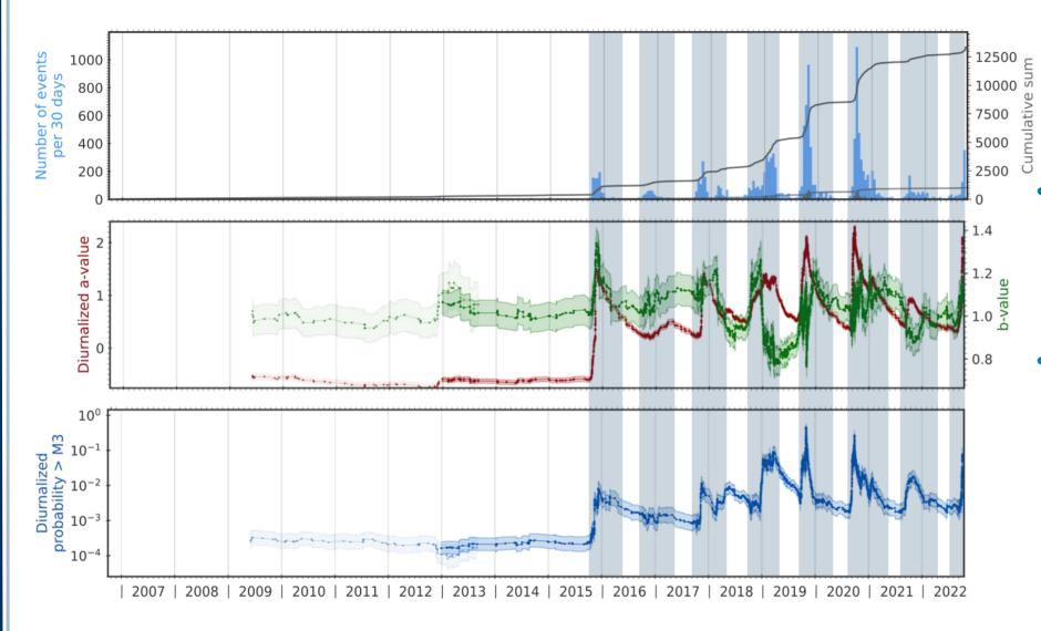
Strong increase in seismic activity in 2015 accompanied by a stronger fluctuation of the three statistical parameters, e.g., higher b-values in fall
