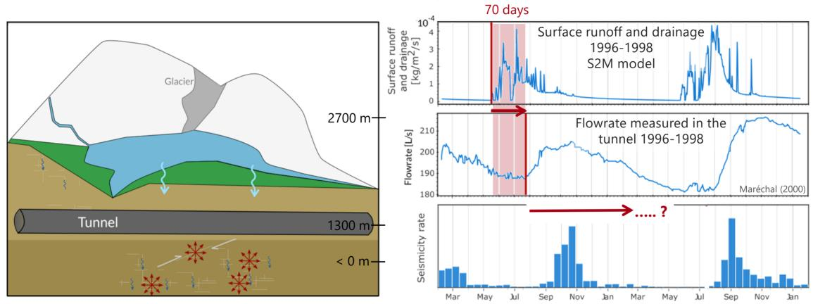
Tracer Tests on Glacier de Toule (Dubois, 1992 and Marechal, 1998): Confirmed the water circulation between the surface and the fracture zone in the tunnel.
