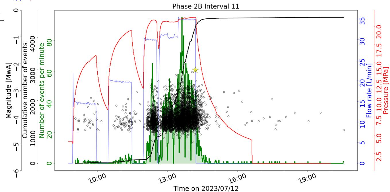
Seismic catalogue creation with python-based open source software
