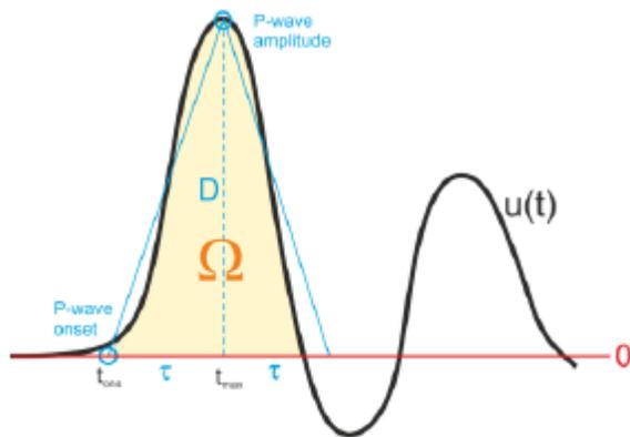
$$\Omega \approx D \tau \text{sgn}(u(t_{\text{max}}))$$
