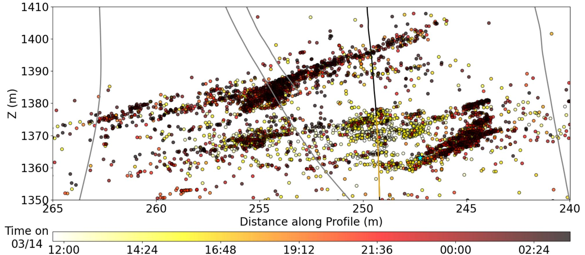
Spatio-temporal evolution of the seismicity along different fractures
