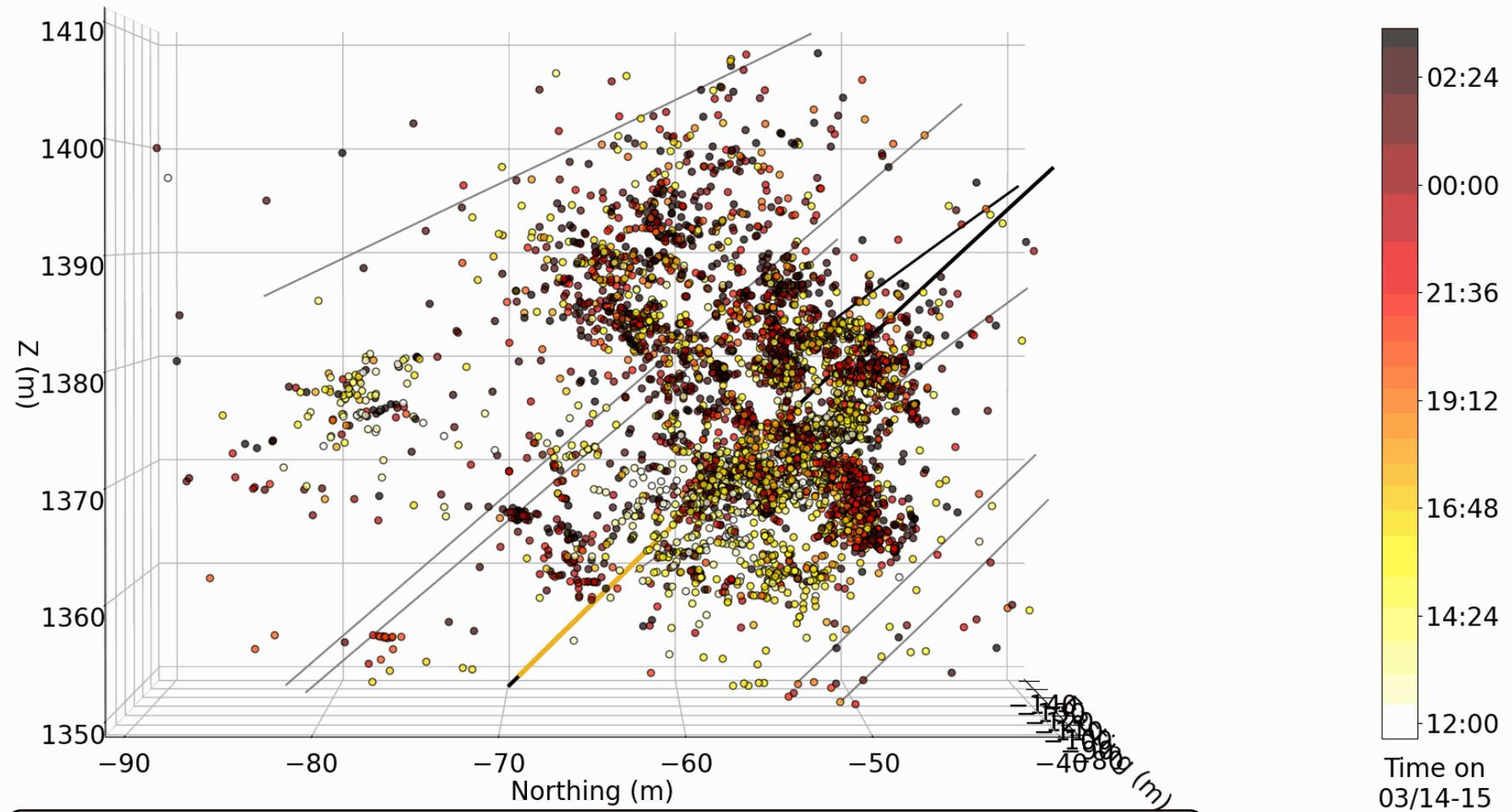
Spatio-temporal evolution of the seismicity along different fractures
