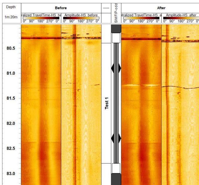
**Fig. 4** Comparison of ATV logs before and after the SIMFIP test. The packer and SIMFIP clamp (black triangle) positions are shown in the middle.
