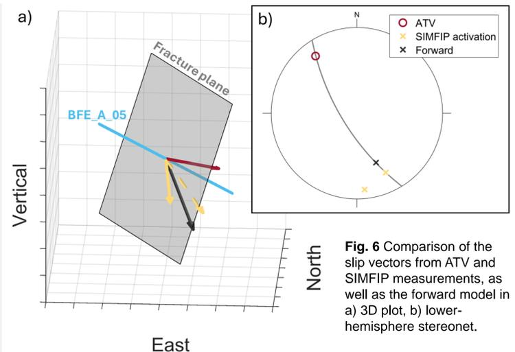
**Fig. 6** Comparison of the slip vectors from ATV and SIMFIP measurements, as well as the forward model in a) 3D plot, b) lower-hemisphere stereonet.
