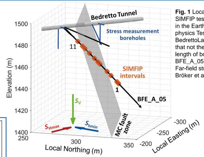
**Fig. 1** Location of the SIMFIP test intervals in the Earthquake physics Testbed at the BedrettoLab. Note that not the full length of borehole BFE\_A\_05 is shown. Far-field stress taken Bröker et al. (2024).
