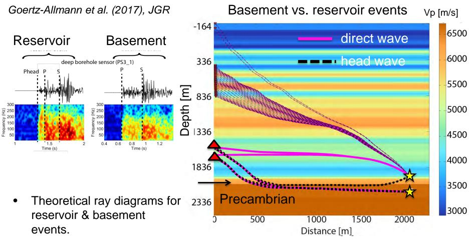
Different waveform signature: head wave and direct wave arrivals clearly visible for reservoir events.
