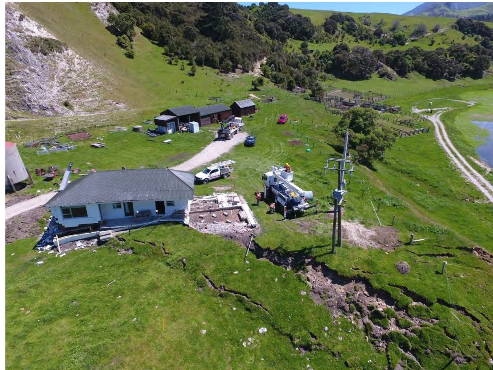
Keekerengu Fault rupture displacement by ~10 meters
