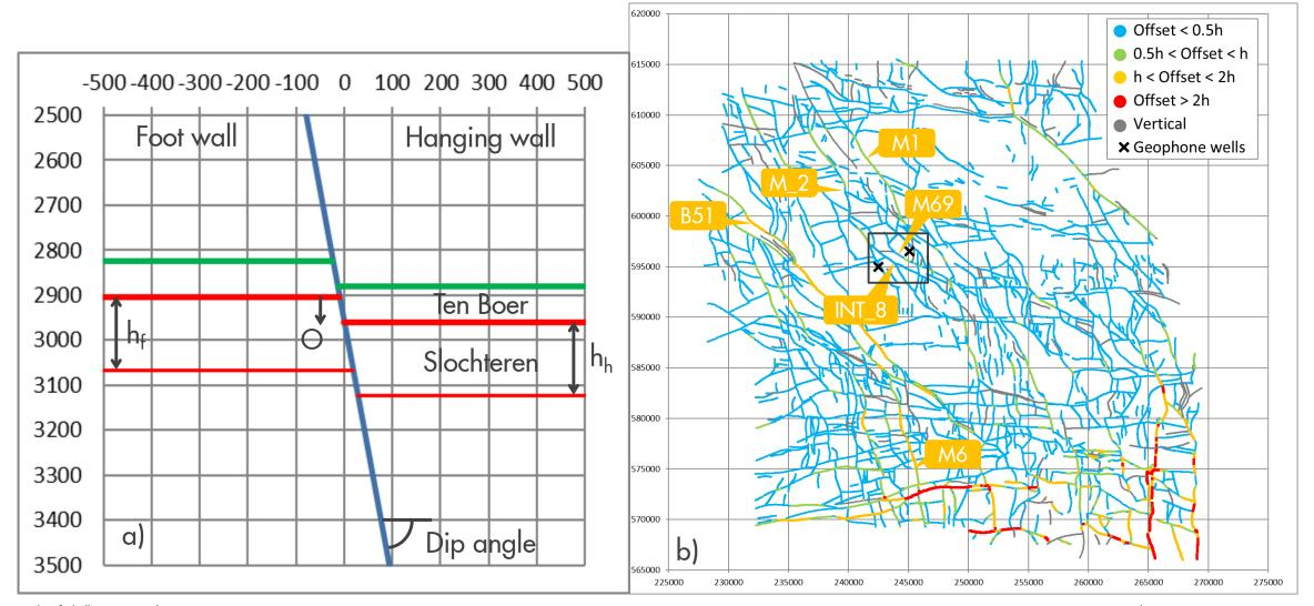
Seismic Rupture is dependent on normalised offset and slope  $\mathbf{W}_{\boldsymbol{\mu}}$
