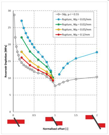
■ Fault reactivation and seismic rupture strongly dependent on normalised reservoir offset
