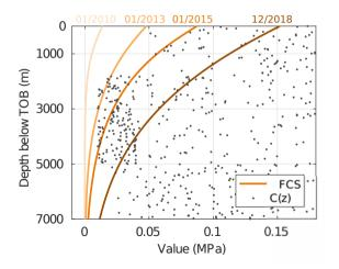
$\Delta FCS(z, t) = 0.5\Delta\sigma_d - \sin\phi_f (\Delta\sigma_m - \Delta p)$ : Change in failure criterion stress
