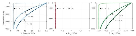
Failure Criterion Stress for optimally oriented faults
