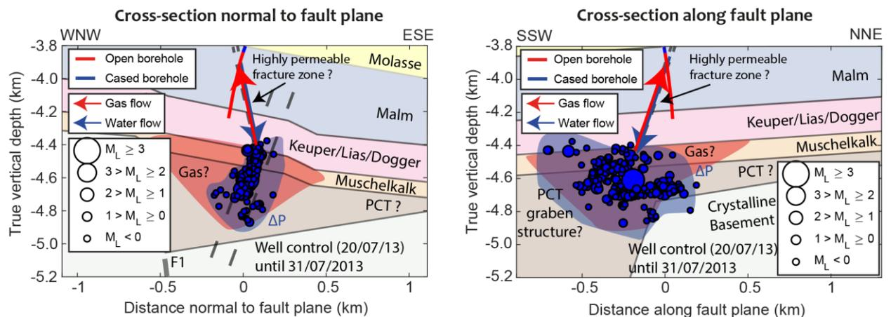
**Fig. 1** Conceptual model of the gas kick and the well control measures: the seismicity is either induced directly by pore pressure increase through a fracture zone or due to poroelastic stress change without any hydraulic connection. The gas kick suggests a hydraulic connection to a source at greater depth.
