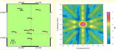
Fig. 7 BURAR sensors distribution (left) and array response (right).
