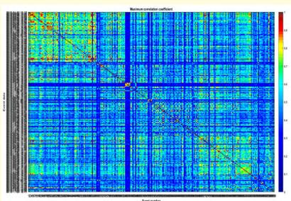
Fig. 15 Correlation matrix for BUR03 recordings filtered using a Butterworth band pass filter between 1 and 10 Hz.
