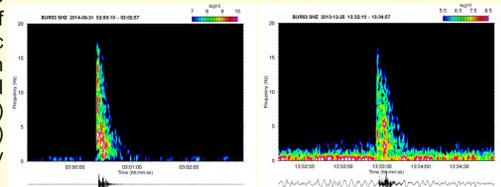
Fig. 8 Spectrograms plots for vertical component of BUR03 station associated to a GT event (left) and an supposed Eq. (right).
