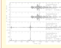
Fig. 5 Example of event detection using cross-correlation algorithm at BURAR seismic array.
