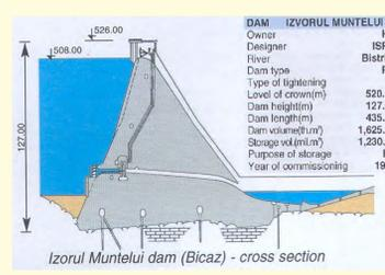
Fig. 4 Cross-section and technical details of the Izvorul Muntelui dam (Cajocar, 2008).
