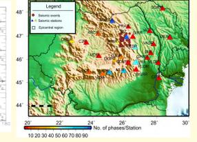
Fig. 6 Stations distribution coloured as the function of data contribution to seismic bulletins.
