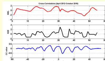
Fig. 17 Cross-correlations values (blue) computed for the normalized time series of water level variation (red) and seismic activity (black).
