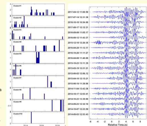
Fig. 16 Clusters of seismic events in time (left) and the waveforms (associated to the 1<sup>st</sup> cluster) recorded by BUR03 station, filtered using a Butterworth band pass filter between 1 and 10Hz.
