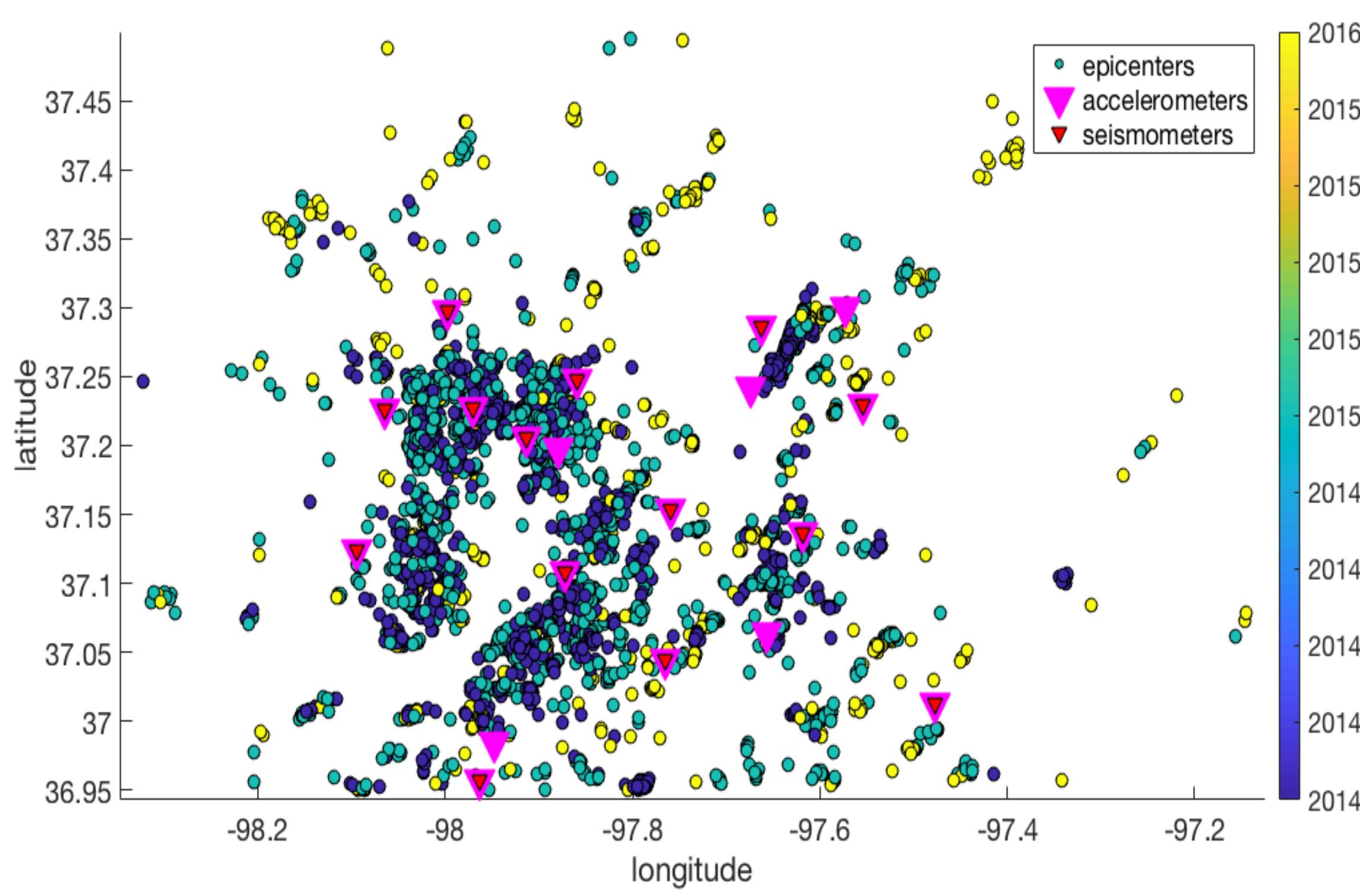
Figure 4: Seismicity map of the 5269 relocated earthquakes (colored with time) recorded by the USGS seismic network.. Seismometers and accelerometers are represented by red and magenta triangles, respectively.
