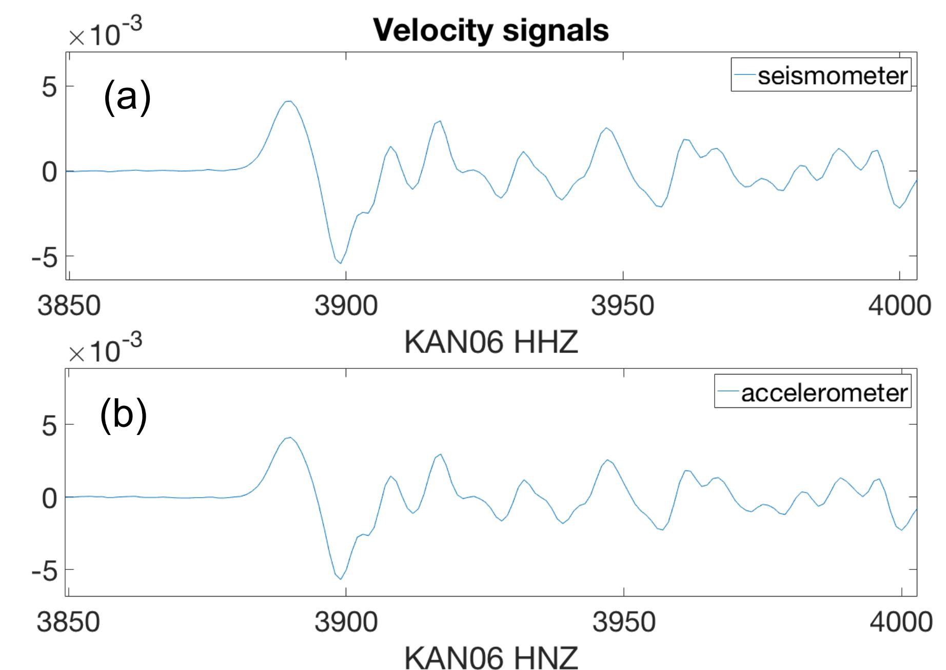
Figure 6: Comparison of the velocity signal between (a) a seismometer and (b) its collocated accelerometer. Polarity and size of the first pulse are similar.
