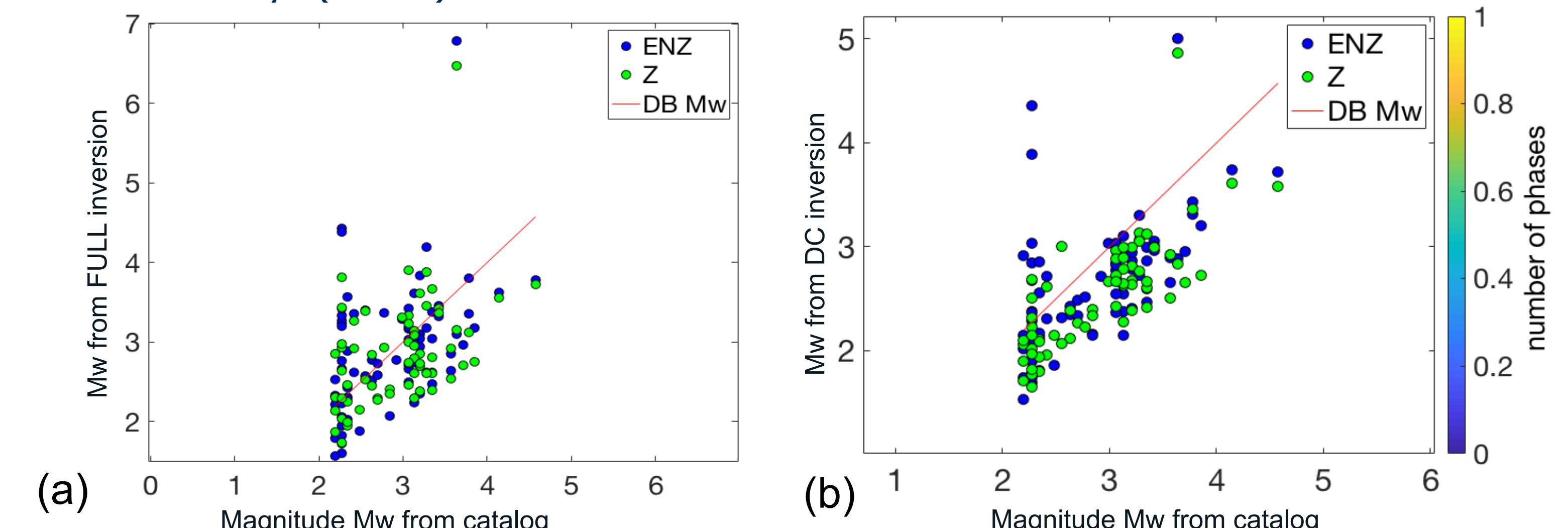
Figure 7: Comparison between the moment magnitude from (a) full inversion, (b) DC inversion and the converted  $M_L$  (to  $M_w$ ) using the scaling from Ref.4 .
