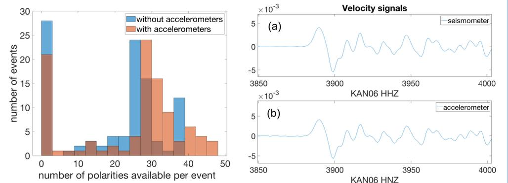
**Figure 5:** Number of manual picked polarities in the test dataset. **Figure 6:** Comparison of the velocity signal between (a) a seismometer and (b) its collocated accelerometer. Polarity and size of the first pulse are similar.
