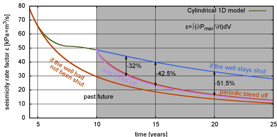
Figure 2: Evolution of seismicity rate factor for various 1D solutions inside a cylindrical reservoir volume  $V$ .
