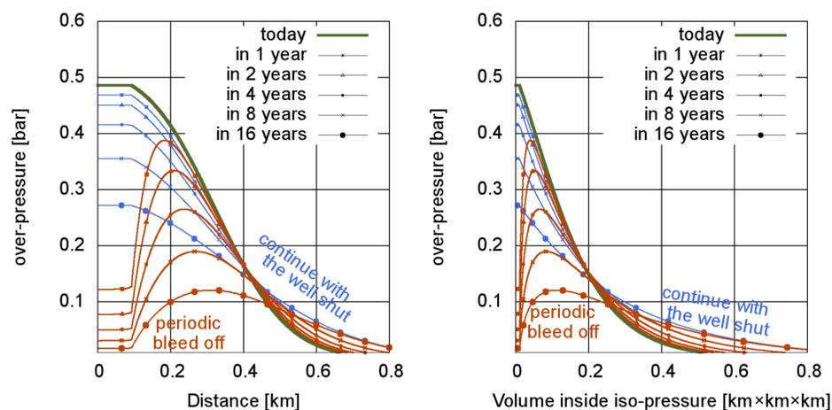
Figure 1: On the left, the estimation of pore pressure changes today and its evolution for two different future scenarios are plotted. On the right, the same results are plotted as a function of the volume size enclosed by each radius.
