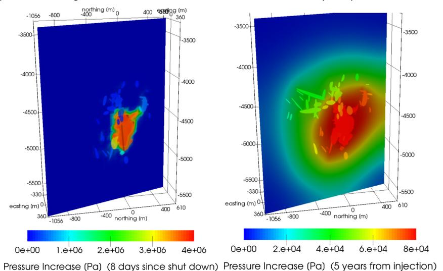
Figure 4: On the left, the distribution of the simulated pore pressure change for the 8th day since the last injection and on the right for the 5th year since the last injection are plotted along a 2D slice of the 3D discrete fracture model.
