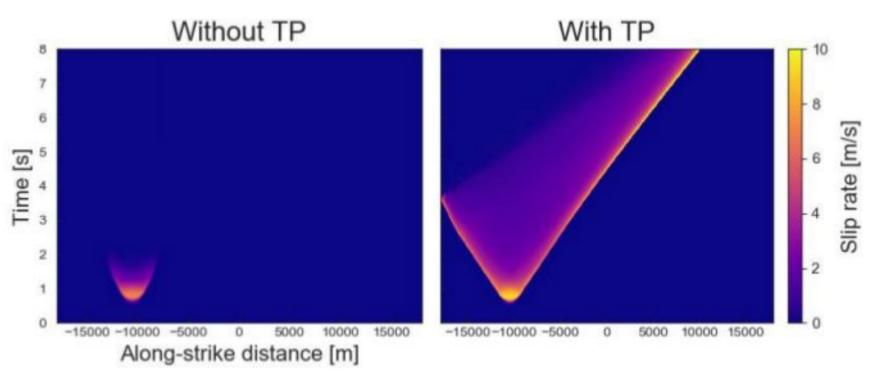
Effect of thermal weakening. Along-strike distance vs. Time with respect to slip rate along a 1D fault in a 2D domain (benchmark by the Southern California Earthquake Center).
