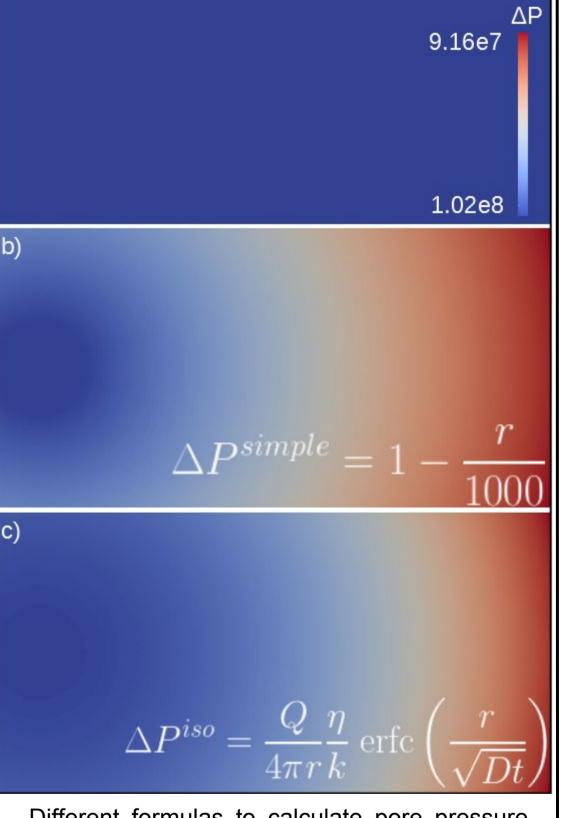
Different formulas to calculate pore pressure gradients. a) constant pore pressure, b) simple pore pressure gradient depending on nucleation size, and c) pore pressure solution in response to injection at a point source in an isotropic, 3D reservoir [3,4].
