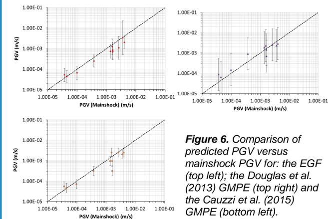
Figure 6. Comparison of predicted PGV versus mainshock PGV for: the EGF (top left); the Douglas et al. (2013) GMPE (top right) and the Cauzzi et al. (2015) GMPE (bottom left).
