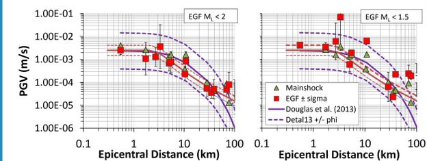
Figure 6. As Figure 4, using only events with M<sub>L</sub> < 2 (left, 46 EGF events) and M<sub>L</sub> < 1.5 (right, 20 EGF events) and showing the GMPEs of Cauzzi et al. (2015) and Douglas et al. (2013).
