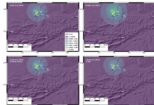
Figure 5. PGV maps (background) and M = 3.2 mainshock amplitude (triangles) for the Basel event. The background maps: the predictions of the Cauzzi et al. GMPE – top left; the predictions of the Douglas et al. GMPE – top right; the interpolation of station records and Cauzzi et al. – bottom left; the interpolation of EGF predictions and Cauzzi et al. – bottom right. The triangles in each map are coloured according to the recorded PGV at each station.
