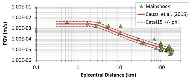
Figure 2. Comparison of the geometrical mean horizontal PGV (for data points where EGF pairs exist) and the GMPE of Cauzzi et al. (2015).
