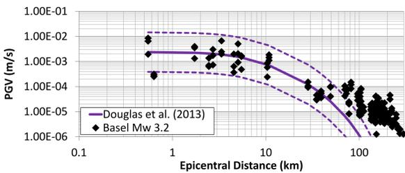
Figure 2. PGV (3-component) from the Basel M = 3.2 event along with the prediction (and plus/minus one within-event standard deviation) from the GMPE of Douglas et al. (2013).
