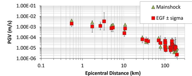
Figure 4. PGV (geometrical mean horizontal) from the Basel M = 3.2 event along with the prediction (and plus/minus one standard deviation) from the EGF predictions.
