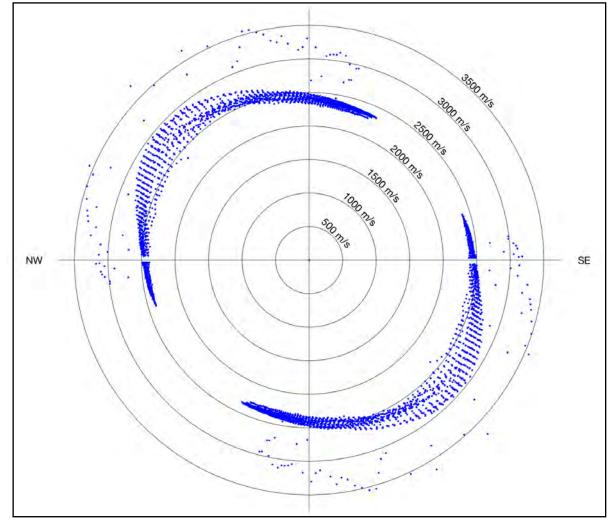
P-wave velocities within a vertical plane, striking NW-SE. This is parallel to the dip of the bedding plane. Note the strong variation of velocity (anisotropy)
