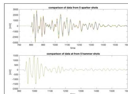
The sparker and especially the hammer sources show an excellent repeatability, which is essential for time-lapse monitoring and imaging.
