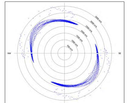
P-wave velocities within a vertical plane, striking NW-SE. This is parallel to the dip of the bedding plane. Note the strong variation of velocity (anisotropy)
