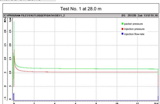
↑ Overnight shut-in test (~14 hours) to obtain formation pore pressure and permeability
