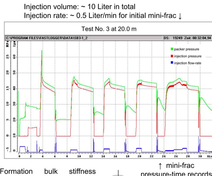
Formation bulk stiffness measurement via dilatometer while conducting dry-packer test to obtain the formation re-opening pressure →
