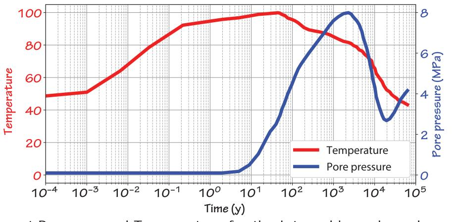
Input Pressure and Temperature for the internal boundary element
