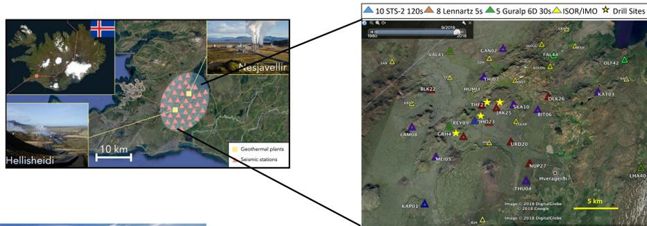
Fig 1. Dense seismic network in the Hengill area installed in October 2018. The yellow stars mark drill sites that are planned to be stimulated later this year.
