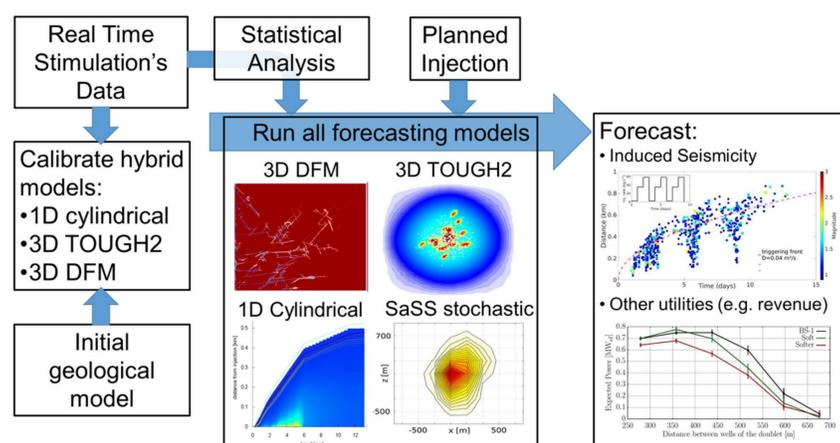
Fig 3. ATLS integrates forecasts both of induced seismicity and of the efficacy of a given injection plan from its suite of models. These models are of varying complexity and take into consideration several observations besides observed seismicity.
