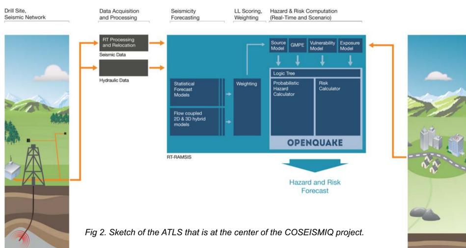
Fig 2. Sketch of the ATLS that is at the center of the COSEISMIQ project.
