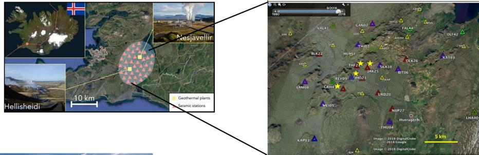
Fig 1. Dense seismic network in the Hengill area installed in October 2018. The yellow stars mark drill sites that are planned to be stimulated later this year.
