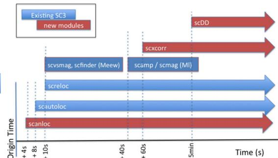
Fig 5. Each new module interacts with existing SC3 modules/information flow. In real-time, scanloc can be expected to work within the ATLS, and results from other modules will be available within minutes of an event and can be revised after manual review, if needed.
