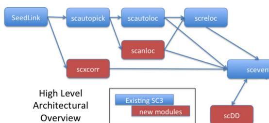
Fig 4. SeisComp3 consists of different modules solving different tasks. Blue rectangles denote standard/existing SC3 modules. Red rectangles denote new (or in development) SC3 modules for real-time induced seismicity monitoring
