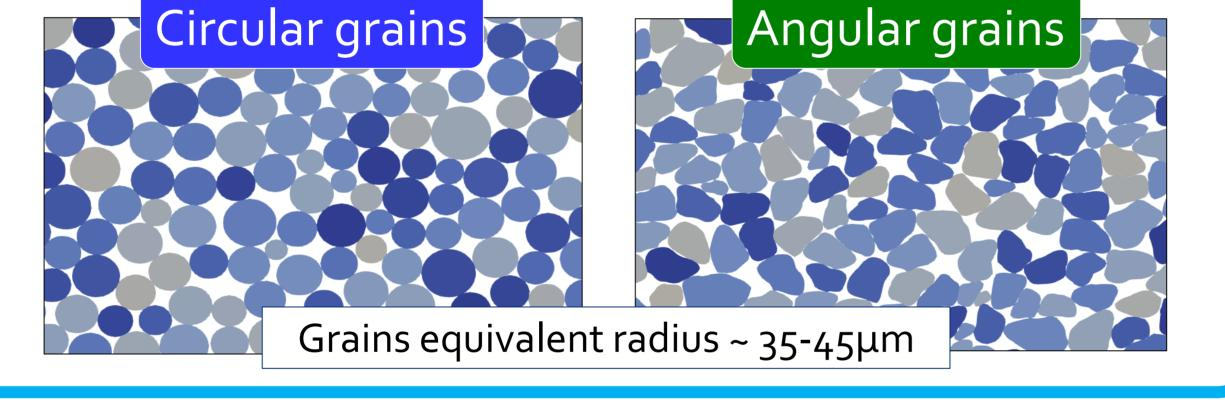
Final position of the grains, color-coded by their initial position.
