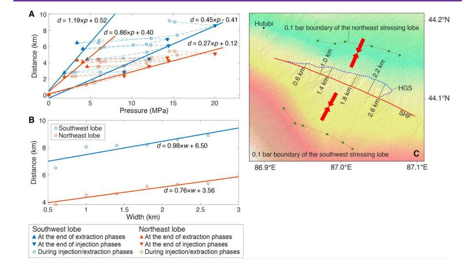
To assess potential seismic hazard, we conducted the simulation to make the HNGR be up to the designed maximum working pressure of 34 MPa.
