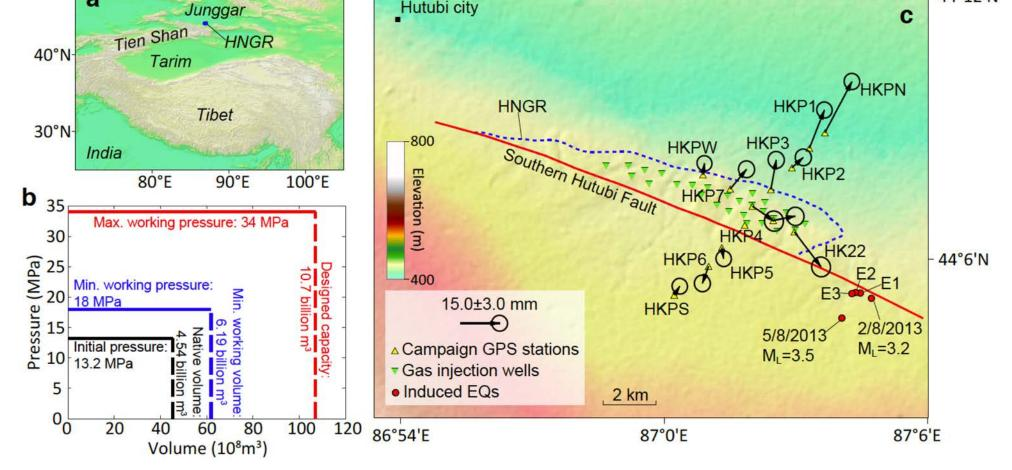
Here, we focus on horizontal GPS observations and make efforts to extract robust displacement signals linked to the cyclic gas injection and extraction of the HNGR. In addition, a hydrogeologic model for the HNGR is built up by using multiple geologic and geophysical data. Fully-coupled poroelastic simulation is conducted to investigate the physical mechanisms of ground displacements and induced seismicity, and also to assess the induced seismic hazard.
