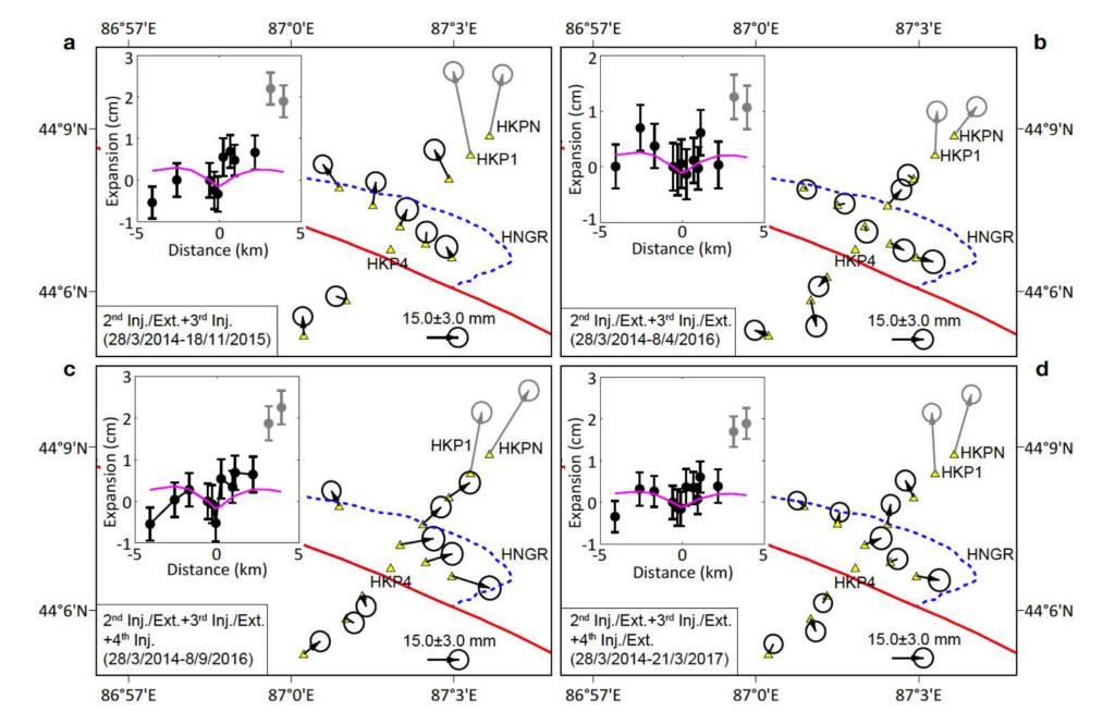
Taking no account of two stations HKP1 and HKPN with extremely large displacements probably contaminated by groundwater extraction, the observed maximum horizontal expansion increases with gas injection phases from 1.02 cm to 1.57 cm, spanning ~1.5, ~2.5, and ~3.5 years, respectively. The other two intervals with equivalent injection and extraction phases (Panel b and d) have a close maximum value of 0.8 cm. The maximum expansion magnitudes correlate with the gas volume changes in the HNGR.
