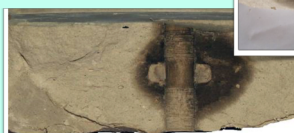
Fig.2. Hydraulic fractures in cross-section view (left) and samples top view after fracturing (right).
