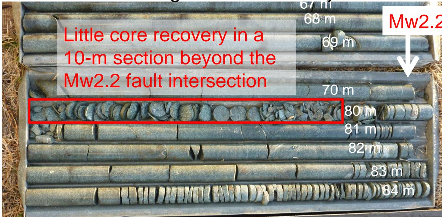
During the following Jpn-SA project (2009-2015), Ogasawara et al. (2012) optimized an overcoring technique suitable for working condition at highly stressed ground in SA gold mine, demonstrating that **core recovery with minimum damage even at earthquake-prone ground is feasible** with great care for drilling direction.
