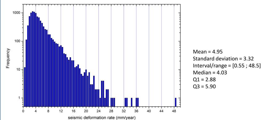
Figure 5 – Histogram of the computed seismic strain and statistical values
