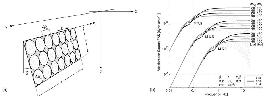
**Figure 2.** (a) Schematic view of Specific Barrier Model, showing fault plane divided into an aggregate of circular cracks. (b) SBM source acceleration spectra for three different magnitudes with varying global ( $\Delta\sigma_g$ ) and local ( $\Delta\sigma_l$ ) stress drop. The associated corner frequencies are marked by large dots. Thin dashed lines include the Kappa filter effect.
