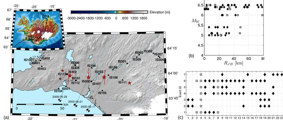
**Figure 1.** (a) Map overview of the study area with stars indicating earthquake epicentres and triangles representing accelerometer stations. (b) Magnitude-distance distribution. (c) Distribution of records indicating which station has accepted data for a given event (rock sites are in black diamonds and soil sites are in grey squares).
