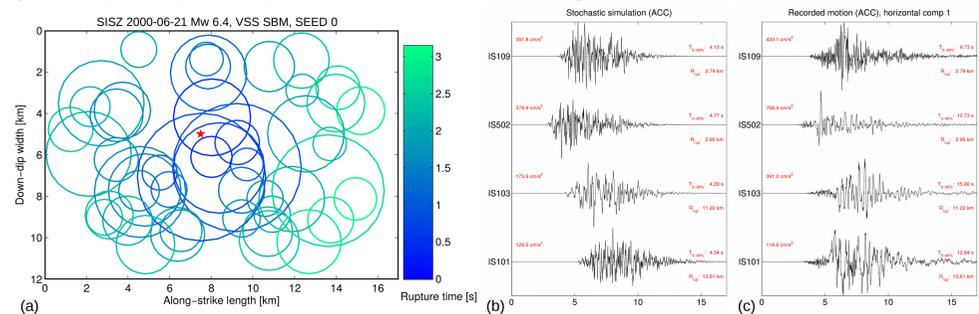
**Figure 4.** (a) Subevent distribution over fault, colored according to their respective rupture initiation times. Also shown are corresponding simulated (b) and recorded (c) ground motions.
