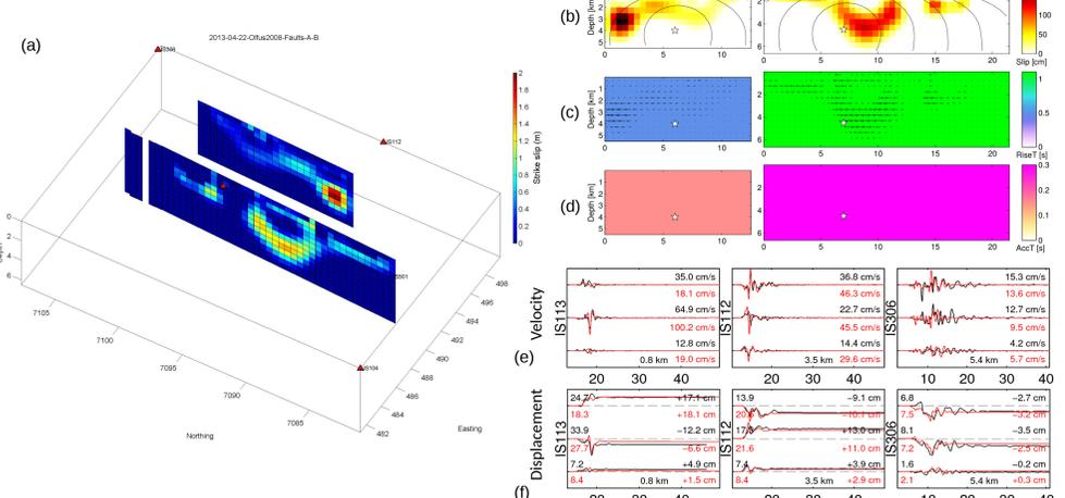
**Figure 5.** (a) 3D representation of the 29 May 2008 earthquake doublet ( $M_W 6.3$ ) from the SISZ. The assumed slip (b), rise time (c) and acceleration time (d) for both fault segments are used to simulate velocity (e) and displacement (f) ground motion (synthetics: red, observed waveforms: black).
