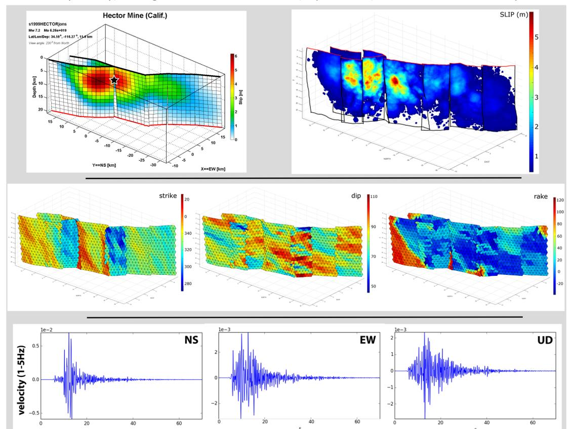
**Figure 3. Top:** input low-resolution (left) and high-resolution slip model (right). **Middle:** strike, dip and rake after fault roughness has been added (a low-resolution mesh is shown). **Bottom:** sample synthetics in the 1-5Hz frequency range (no low-frequency component).
