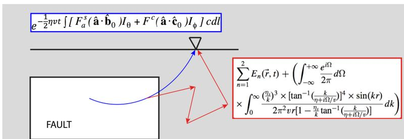
**Figure 1.** Sketch illustrating the double nature of the high-frequency radiation (S-waves case): deterministic (in blue) and stochastic (in red). The deterministic component (obtained by calculating surfaces integrals on the fault plane) is attenuated by the frequency-dependent exponential term. The energy lost by scattering is transferred to the stochastic component, whose envelope is controlled by the multiple S-to-S scattering model (red box).
