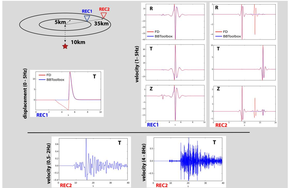
**Figure 2. Top:** comparison between synthetic seismograms computed using our code (in blue) and a finite-difference (FD) code (in red). Note the presence of an evanescent P-wave for receiver 2 in the FD solution. **Bottom left:** displacement on the transversal component for receiver 1, evidencing the near-field motion missing in our solution. **Bottom:** synthetics at two different frequency bands for receiver 2, this time including scattering attenuation.
