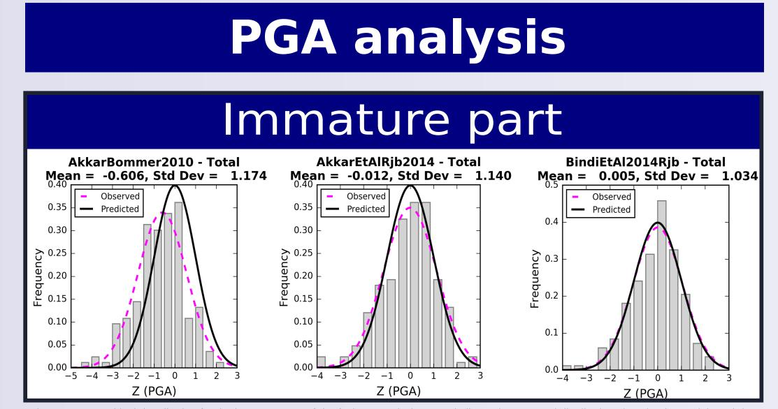
Figure 3: PGA residual dostribution for the immature part of the fault zone. Black curves indicate the expected distribution given by the models and the
