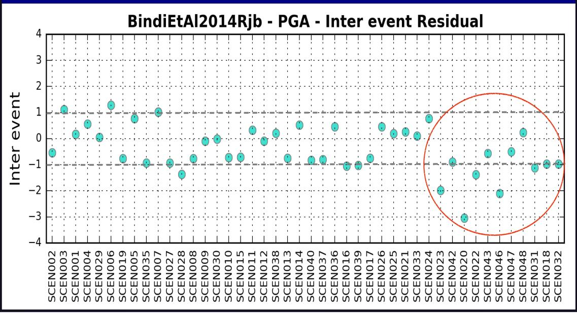
jure 7: The source-specific residual analysis shows the residuals for the reference model of Bindi et al., 2014 for the entire dataset (sorted by their longitude increasing m west to east).The red circle shows the residuals only for the mature part, which are out of range with respect to the ground motion model.
