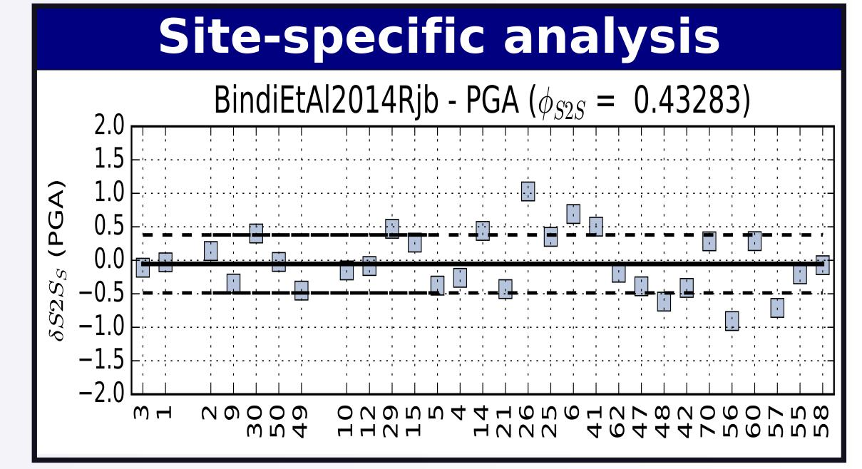
Figure 8: Site-specific within-event residual analysis for each station. The blue squares represent the averaged within-event residual for each site. The sites are sorted by their longitude. Stations until 26 are all located on the immature part of the fault zone.
