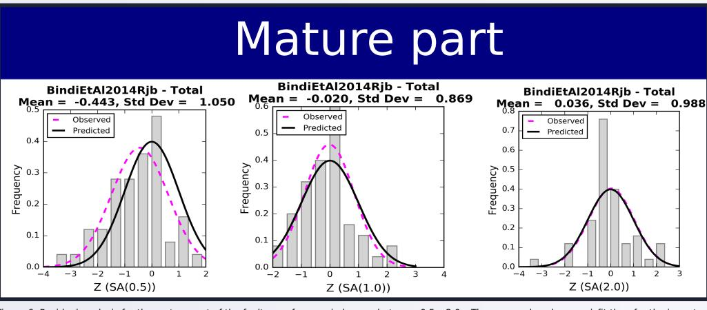
Figure 6: Residual analysis for the mature part of the fault zone for a period range between 0.5s- 2.0s. The curves show larger misfit than for the immature part
