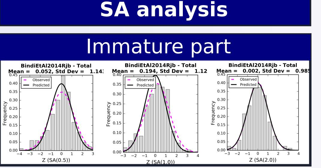
Figure 5: Residual analysis for the pseudo-spectral acceleration for a period range between 0.5s - 2.0s. The curves show a perfect fit to the observed data for a
