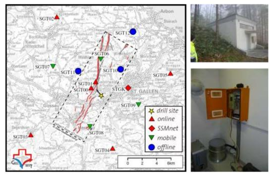
**Figure 5:** Left: Map of the St. Gallen region where symbols show the locations of sensors installed by the SED to monitor the St. Gallen hydrothermal project. Right: Example of a seismic station installation.
