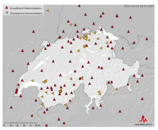
**Figure 3**: Map of the Swiss Digital Seismic Network (SDSNet) as of October 2017. All seismological broad-band (red triangles) and short-period seismometers (yellow left arrows) that are recorded in real-time at the SED data centre in Zurich are indicated. An updated version of this map can be found on the SED web page<sup>9</sup>.
