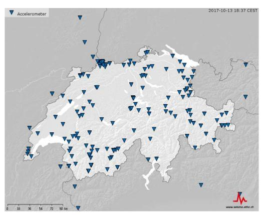
**Figure 4**: Map of the Swiss Strong Motion Network (SSMNet) as of October 2017. All accelerometer station (blue inverted triangles) that are recorded in real-time at the SED data centre in Zurich are indicated. An updated version of this map can be found on the SED web page<sup>10</sup>.
