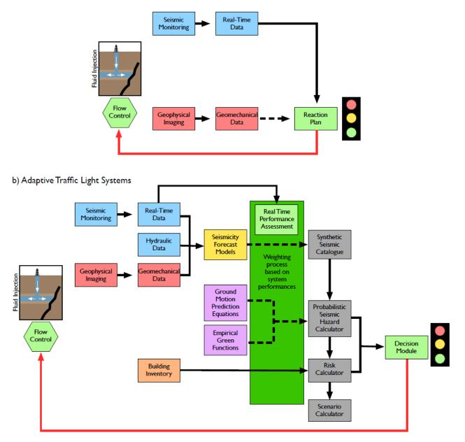
**Figure 31:** a) Classical Traffic Light System. Decisions are based on observed magnitudes and ground motions. Thresholds are defined in a static manner taking geotechnical information into account to the extent possible. b) Proposed Advanced Traffic Light System. Decisions are based on a forward looking, probabilistic and adaptive framework. Models are assessed in near real time and weighted accordingly. After Grigoli et al. (2017).
