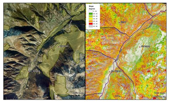
Figure 4: Detail of deposits and inclination for the area of St. Niklaus / Grächen / Embd.
