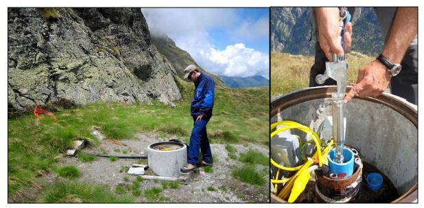
**Figure 8**: Borehole sb120 at Randa, showing the surrounding area and borehole top, and detail of the inclinometer casing and in-place inclinometer instrument.
