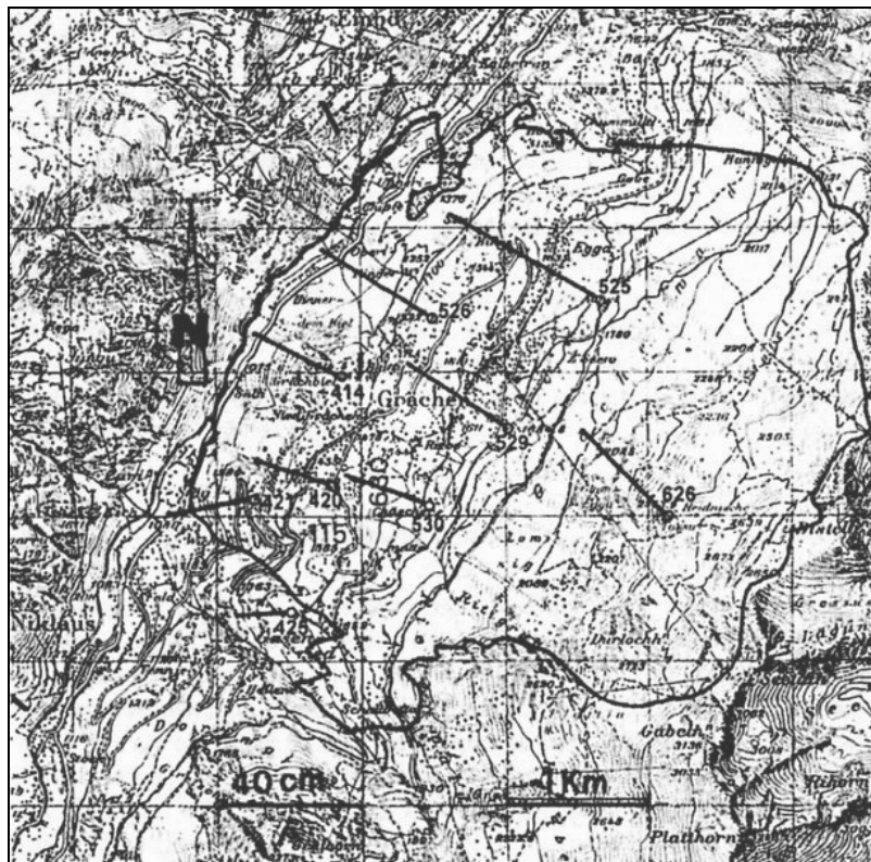
Figure 18: Graechen geodetic monitoring overview. Displacement vectors were calculated over a 62 year period from 1930-1992, and are scaled according to the legend in the lower left portion of the map. Figure reproduced from Noverraz et al. (1998).
