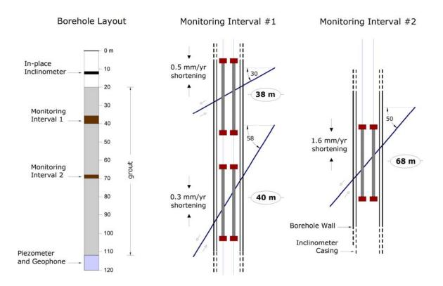
**Figure 2:** Detail of fiber optic sensor installation in borehole *sb120*. Two monitoring intervals were selected to span three active fractures showing normal mode offset (see slip arrows). The expected rates of shortening, calculated from previous extensometer surveys, are shown. Two active parallel sensor chains were installed for redundancy and security, and a third inactive chain (not shown) acts as reserve.
