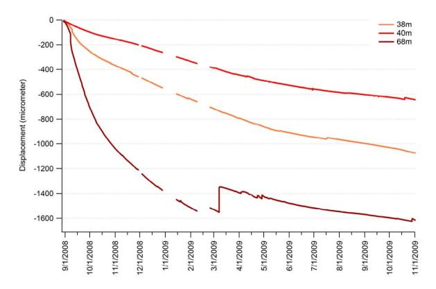
**Figure 3:** Deformation time series measurements from the three sensors at different monitoring intervals in borehole sb120 (data from just one sensor chain are shown). All sensors are shortening as expected. Accelerated shortening is seen immediately following sensor installation, which likely results from shrinkage of the grout. A number of transient steps and drops occur throughout the time history; one event from April 28, 2009 is highlighted in Figure 5. Dates are m/d/y.
