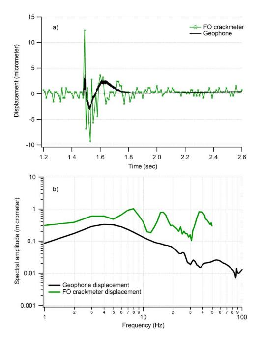
**Figure 8:** Dynamic test results: a) Time history of a shot at 2 m distance comparing the fiber optic crackmeter and the geophone ground motion response; b) Spectra for the same time interval. Low-frequency signals are represented fairly well by the fiber optic sensor, but the fiber optic record suffers from aliasing of higher frequency energy (greater than 50 Hz), which generates an apparent ringing in the time history and false spectral peaks not related to ground motion.
