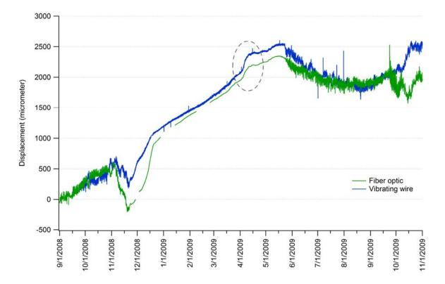
**Figure 6:** Unfiltered fiber optic crackmeter data compared with the time series from the traditional vibrating wire instrument. There is generally good match between the two sensor types, with very similar long-term displacement trends. Some differences likely arise from each sensor's thermal response and the applied temperature correction. The brief acceleration in April is circled and a select portion shown in detail in Figure 7. Dates are m/d/y.
