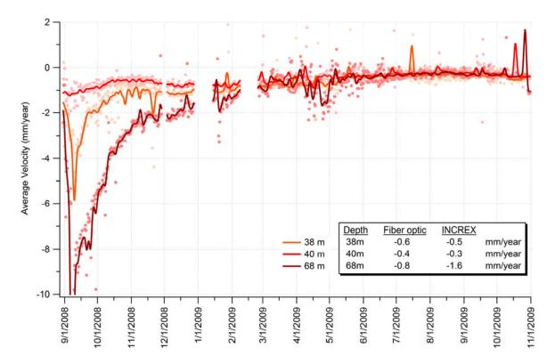
**Figure 4:** Velocity time series for the different sensors in borehole sb120. Dots indicate calculated half-day average velocities, while the solid lines are the data filtered with a binomial smoothing algorithm. The inset table shows comparison of the long-term average velocities with those determined from previous INCREX extensometer surveys. Accelerated shortening is clearly visible in the first 2-3 months of operation. Dates are m/d/y.
