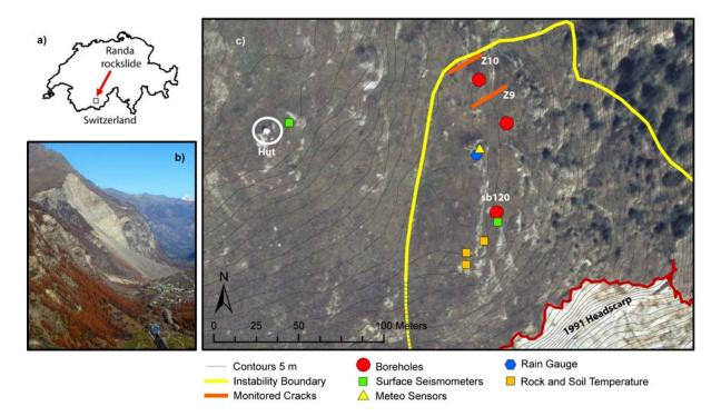
**Figure 1:** a) Location of the Randa rockslide, b) Overview of the rockslide and deposit in the Matter valley, c) Layout of the fiber optic strain sensors (borehole sb120, and cracks Z9 and Z10) and supporting sensors at the top of the currently unstable rock mass. For more details on the structure and kinematics of the unstable rock mass, see Willenberg et al., 2008a,b and Gischig et al., 2009.
