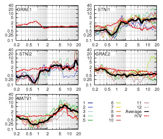
Figure 8: Comparison of average site-to-reference spectral ratios (black thick) for earthquake recordings with H/V curves (dashed red) from ambient noise for the Matter valley area. GRAE1 was the reference station. Colours distinguish between different events.
