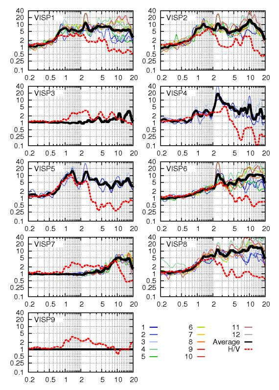
Figure 7:Comparison of average site-to-reference spectral ratios (black thick) for earthquake recordings with H/V curves (dashed red) from ambient noise for the Visp area. VISP9 was the reference station. Colours distinguish between different events.
