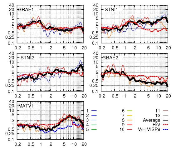
Figure 9: Comparison of average site-to-reference spectral ratios (black thick) for earthquake recordings with H/V curves (dashed red) from ambient noise for the Matter valley area. VISP9 was the reference station. Colours distinguish between different events. V/H ratio for the VISP9 station (dashed blue) is supplied for MATV1 plot.
