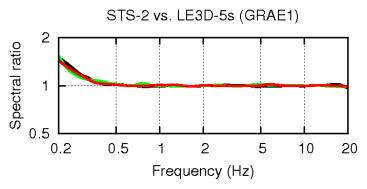
Figure 6: Spectral ratio (STS-2 / LE3D-5s) at site GRAE1 for three events of winter 07/08.
