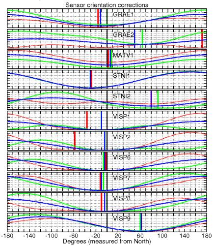
Figure 5:Relative misfit between horizontal components of outside and inside sensors depending on the rotation of the inside sensor (North component – red, East component – green, absolute horizontal component – blue). Colorful vertical bar denotes global minimum of the corresponding curve.
