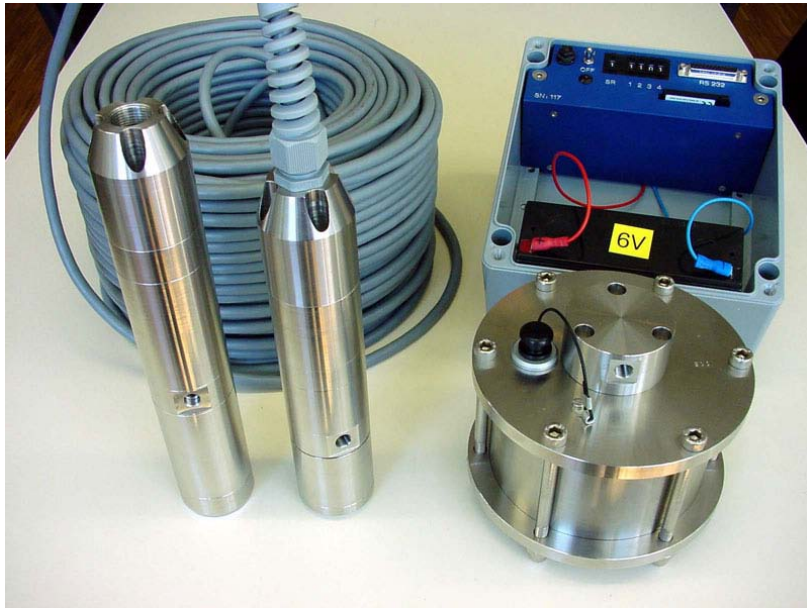
Fig. 6 The GGUN-FL30 flow-through field fluorometer
