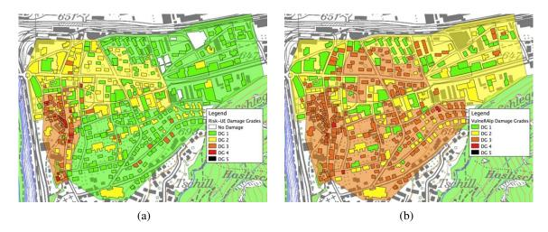
Figure 6: Damage Grades in case of Intensity *VIII* earthquake of the city of Visp according to the (a) Risk-UE LM1 and (b) VulneRAlp methods.
