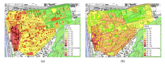
Figure 5: Vulnerability Index (VI) of the city of Visp according to the (a) Risk-UE LM1 and (b) VulneRAlp methods.
