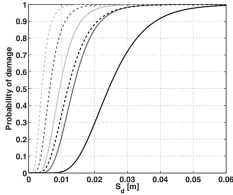
Figure 20: Example of resulting fragility curves for DG 1 (dashed lines) and DG 5 (solid lines) between 3 (light grey) and 5 (black) storeys.
