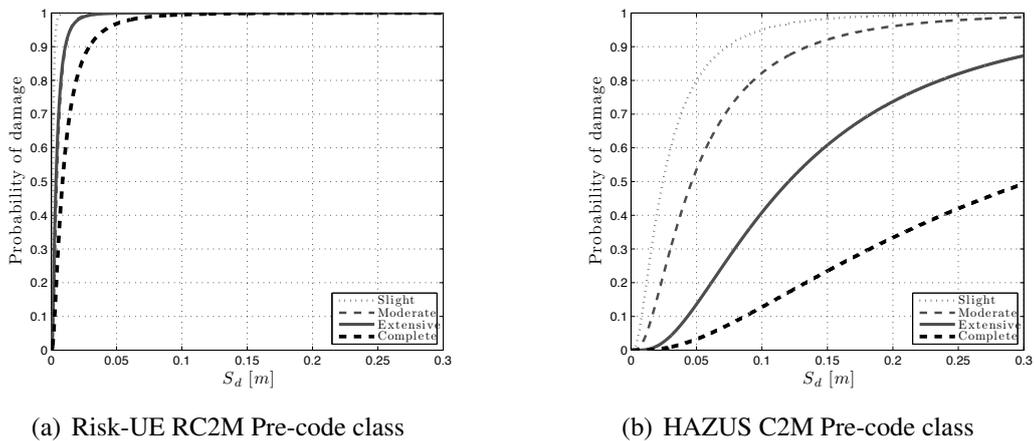
Figure 23: Fragility curves of RC shear wall class from 4 to 7 floors from European and US literature.
