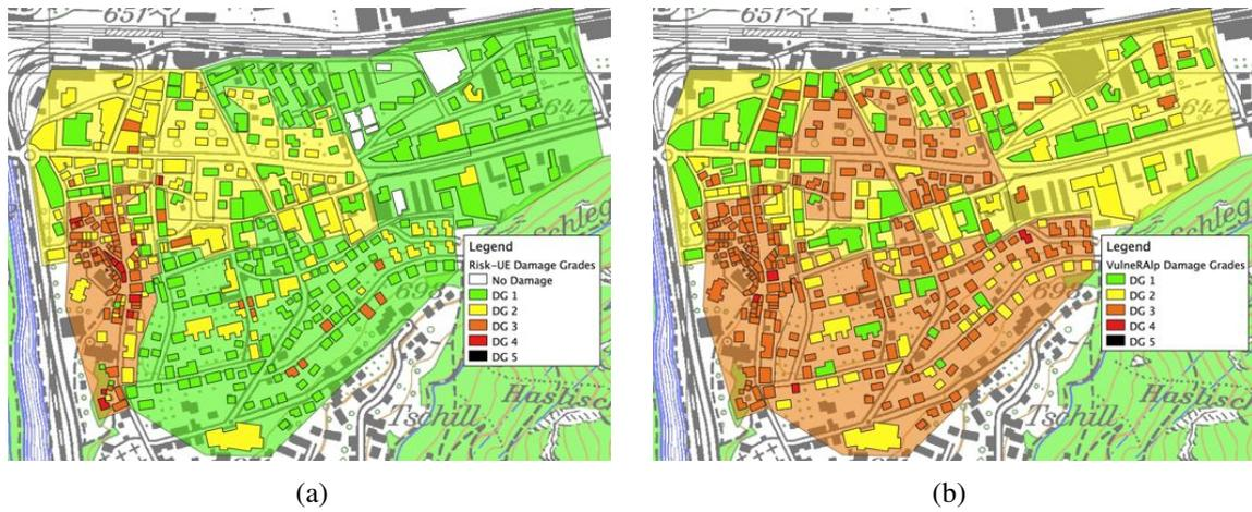
Figure 6: Damage Grades in case of Intensity VIII earthquake of the city of Visp according to the (a) Risk-UE LM1 and (b) VulneRAIp methods.
