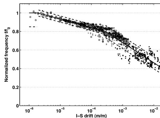
Figure 18: Frequency drop relationship found for clay masonry with the 80% confidence interval.
