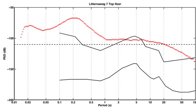
Figure 17: Spectrum of a top floor noise recording in transverse direction in building #9 (Litternaweg 7) in red and comparison with Episensor resolution (dashed black line) and the high and low noise models (solid black lines).
