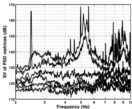
Figure 14: Average FDD spectrum of the recordings in building #2 (Courthouse).
