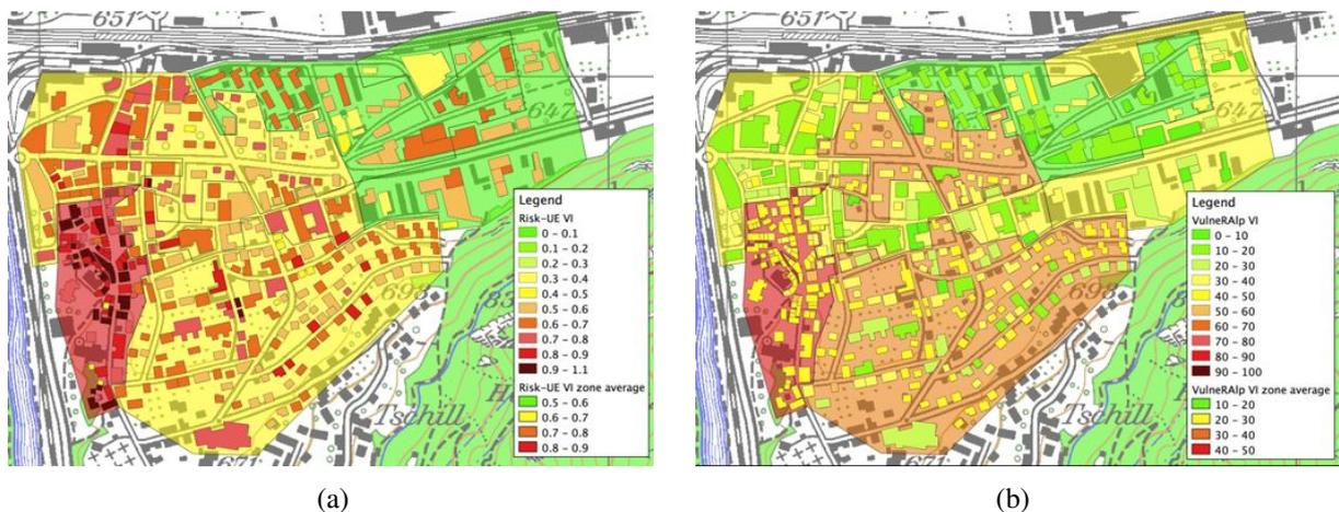
Figure 5: Vulnerability Index (VI) of the city of Visp according to the (a) Risk-UE LM1 and (b) VulneRAIp methods.
