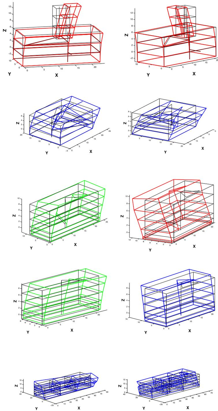
Figure 15: Estimated modal shapes of the first longitudinal and transverse modes of Visp buildings #2, 3, 9, 10 and 18.
