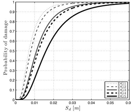
Figure 21: Proposed fragility curves for masonry buildings with stiff floors of 3 to 5 stories.
