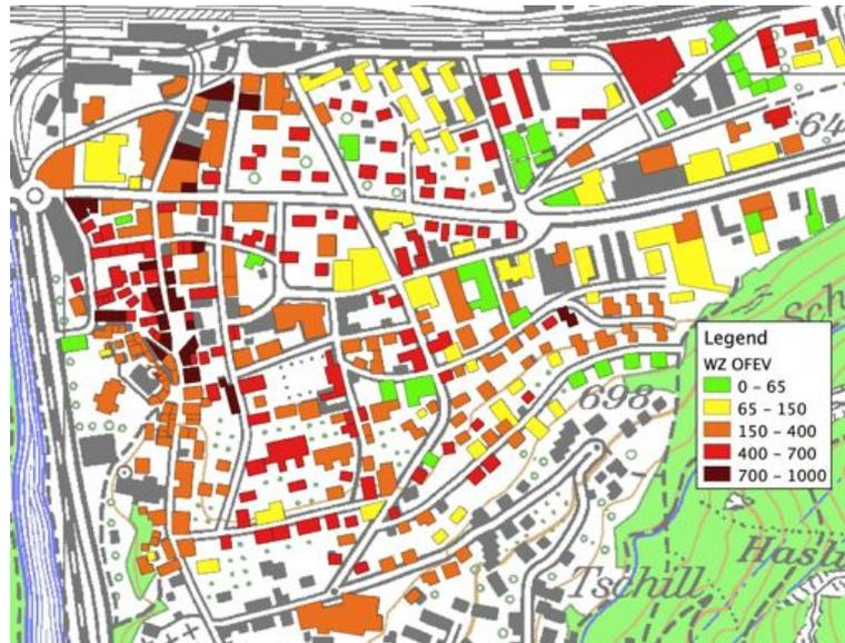
Figure 8: Collapse probability (WZ) of the city of Visp according to the OFEV sorting method.
