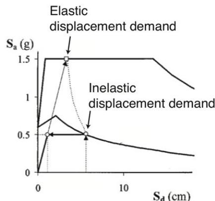
Figure 19: Difference between the inelastic displacement (used as abscissa of the fragility curves in current methods such as FEMA [2003]) and the elastic displacement (used in method 2) following Fajfar [1999] method. From Fajfar [1999].
