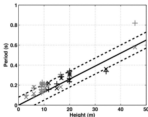
Figure 16: Periods of the study-buildings as a function of building height compared to the relationship found on RC wall structures with its standard deviation. Grey and black stand for masonry and RC structures, respectively. Plus and cross symbols stand for transverse and longitudinal directions, respectively.
