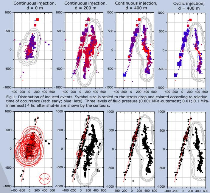
Fig.1: Distribution of induced events. Symbol size is scaled to the stress drop and colored according to relative time of occurrence (red: early; blue: late). Three levels of fluid pressure (0.001 MPa-outermost; 0.01; 0.1 MPa-innermost) 4 hr. after shut-in are shown by the contours.
